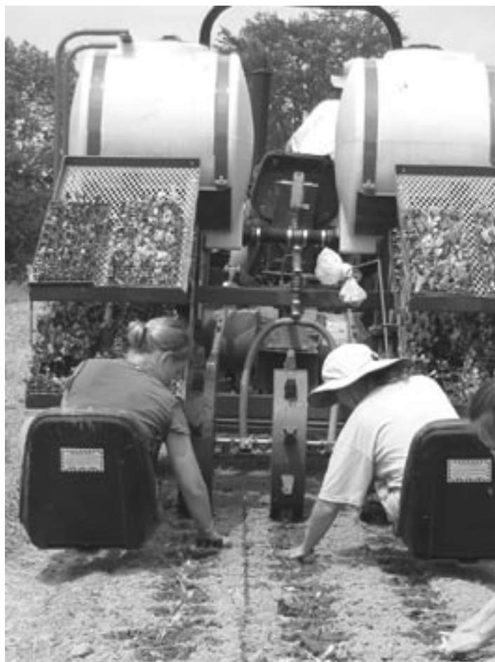
Transplanter purchased with a Ritchie Foundation grant award has improved the efficiency of planting seedlings by 100%!
